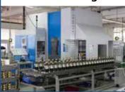
Gear hobbing, gear shaping and broaching / straight-toothed and helical components
