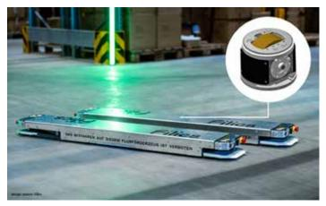
With its innovative dual-runner system, Filics is setting new standards in pallet transport. Framo Morat's ultra-compact drive units deliver exceptional efficiency, handling loads of up to 800 kg at speeds of 1.2 m/s. The system's omnidirectional control and unique pass-through function enable seamless maneuverability, optimizing warehouse automation and ensuring a smooth, efficient material flow.
