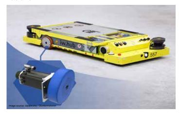
The iw.hub from idealworks, developed in collaboration with Dunkermotoren, leverages Framo Morat's high-performance hub gears for maximum efficiency. With a load capacity of 1,000 kg and a speed of 2.2 m/s, this autonomous underslung AMR ensures precise and reliable material flow. Its compact design and exceptional maneuverability make the iw.hub the ideal solution for in-house transport of pallets and mesh boxes.
