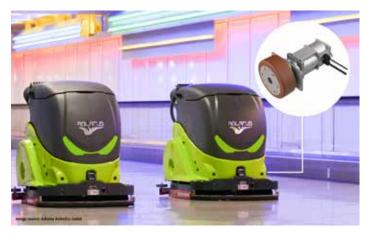
The RNA250 wheel hub drives provide powerful and reliable propulsion for the fully autonomous Adlatus CR700 cleaning robot. With a compact design, a two-stage gearbox, and a load capacity of up to 250 kg per wheel, they are designed for continuous operation in demanding environments.
