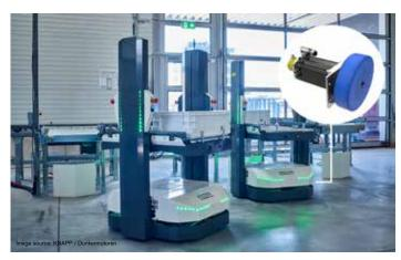
The KNAPP Open Shuttle relies on Framo Morat's NG500 hub gear and the BG 75 BLDC motor from Dunkermotoren. With a 160 mm wheel diameter, high load capacity, and optimized gear kinematics, the drive unit ensures powerful acceleration, precise maneuvering, and a reliable material flow.
